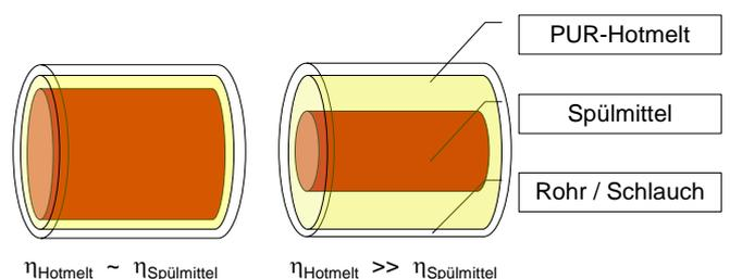
When choosing a Flushing Agent, it is important that the viscosity range of the Flushing Agent is similar to that of the PUR hot melt adhesive (see figure above).
