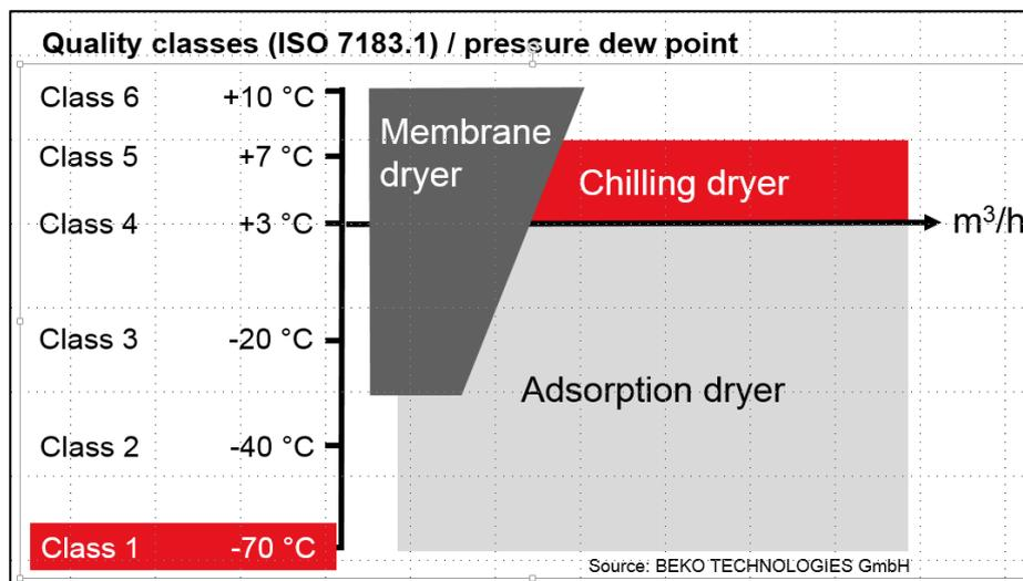
To our knowledge, the somewhat less expensive chilling and membrane dryers are not suitable for producing dry air in the required quality. The water content of the dry air produced by these units is far above the level of 5 ppm, and leads to problems in practical use.
