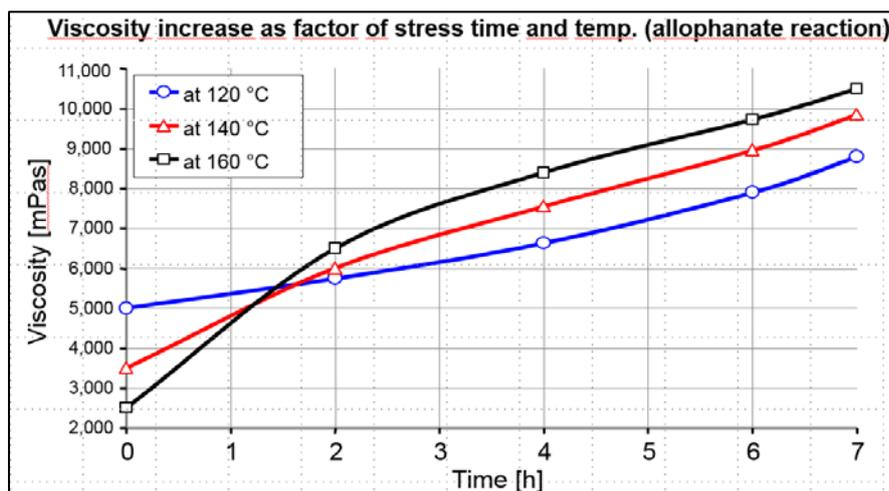
recommended processing temperature, or thermal exposure over a longer period of time, the melt viscosity may increase due to a crosslinking reaction within the adhesive (allophanate reaction) - even if no moisture is present - just due to the influence of the high temperature.
