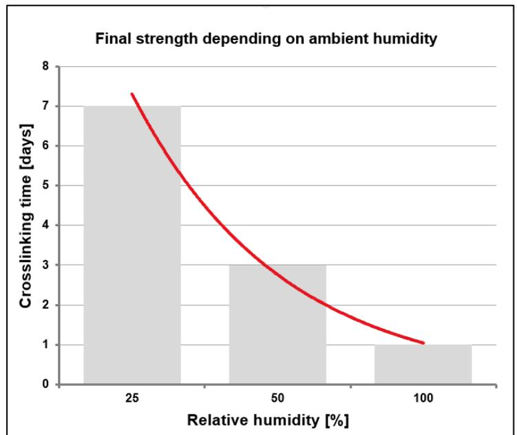
The crosslinking is caused by humidity in the air, and/or moisture contained in the materials to be bonded. Accordingly, the PUR hot melt adhesives have to be protected from any contact with humidity during manufacture, storage and processing, to avoid premature reaction.
