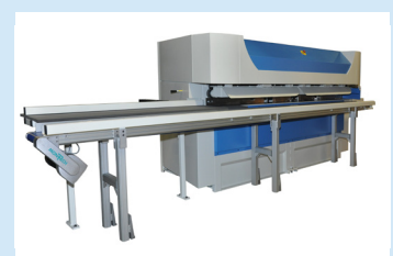
Automatic timber return system
